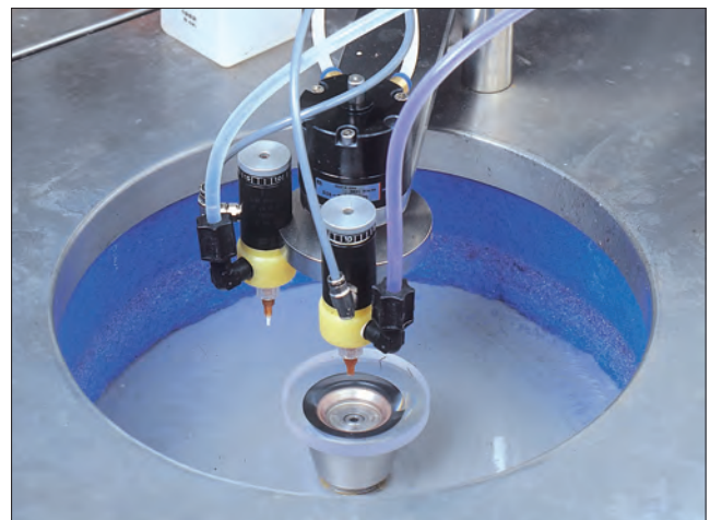
B. Spin Hardcoat application - Concave surface
