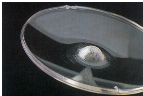
Fig. B "Bullseye Lens" Impact made by an 8mm steel ball travelling at over 90mph.
